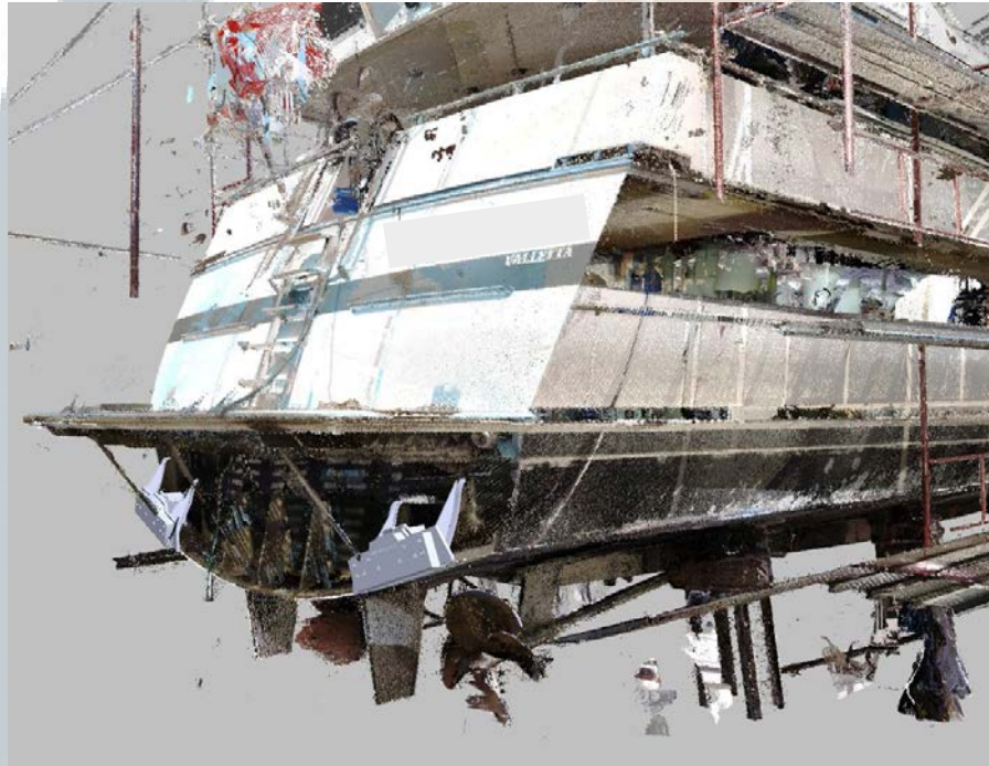
Stabilizer installation on a 29.6m yacht
